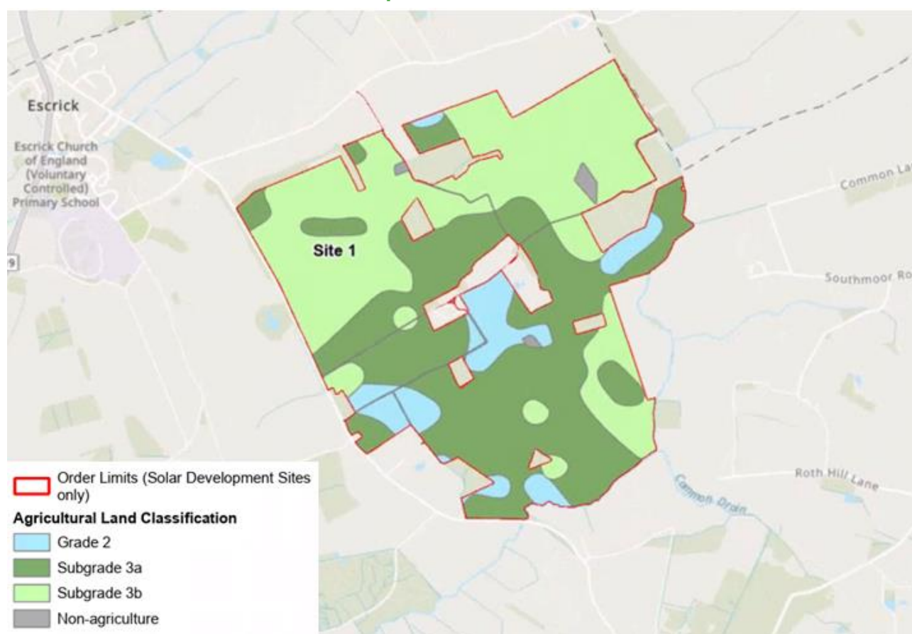
Plate 5-1 ALC in Solar Development Site 1
